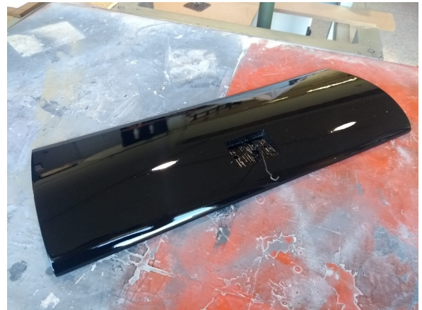
(b) The Airfoil after being sanded and assembled
