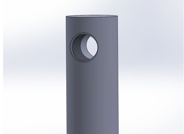
(b) Detail of the rod for fitting to the plate with a screw
