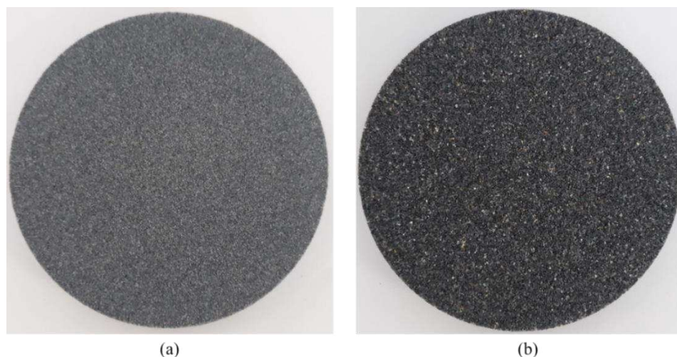
Figure 3.3: Superficial view of the (a) 50 \mu\text{m} and (b) 120 \mu\text{m} porous ceramic filters.
