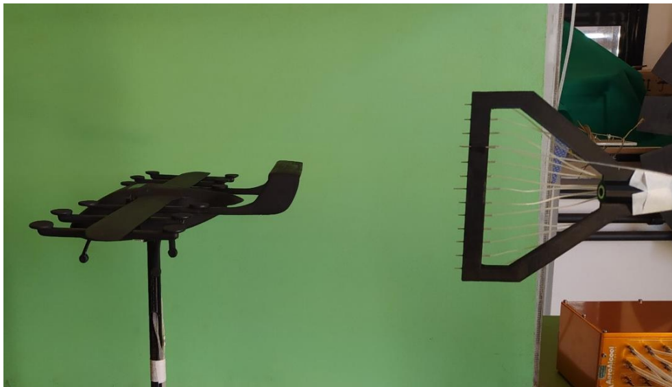
Figure 3.21: Rake positioned right behind the model.
