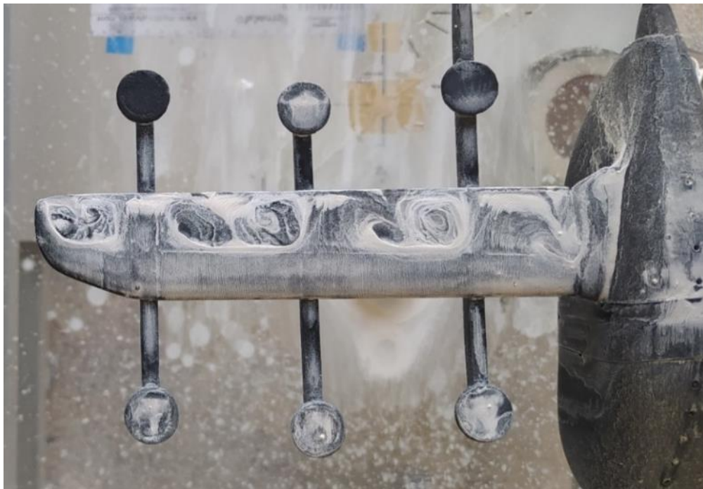
Figure 4.5: Third result of the flow visualization over the wing.
