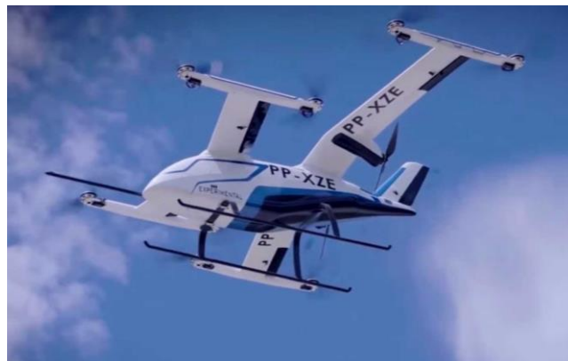
Figure 2.9: Embraer EVE subscale demonstrator.
