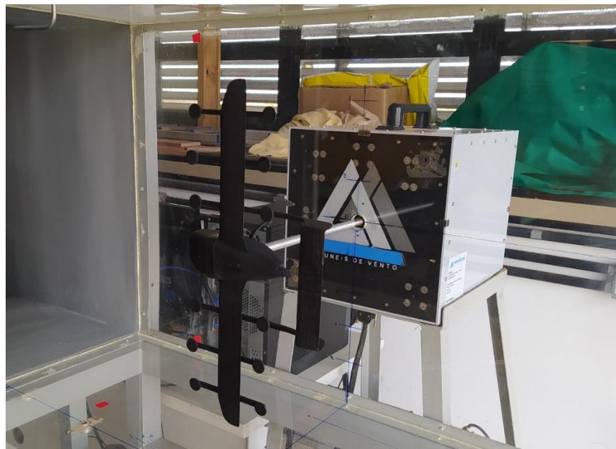
Figure 3.24: Model positioning for the aerodynamic drag evaluation.
