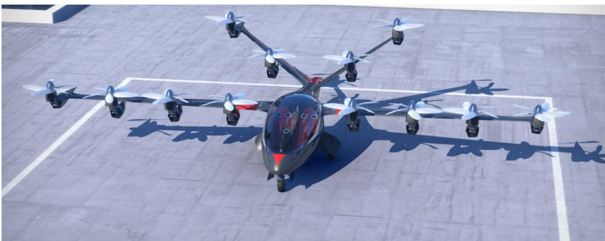
Figure 1.3: eVTOL concept “Joby S2” (defunct), which presented DEP system.
