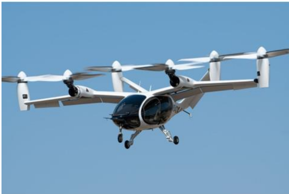
Figure 2.12: The Joby S4 in VTOL configuration.
