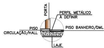
○ DETALHE 01— PERFIL METÁLICO SEM ESCALA
