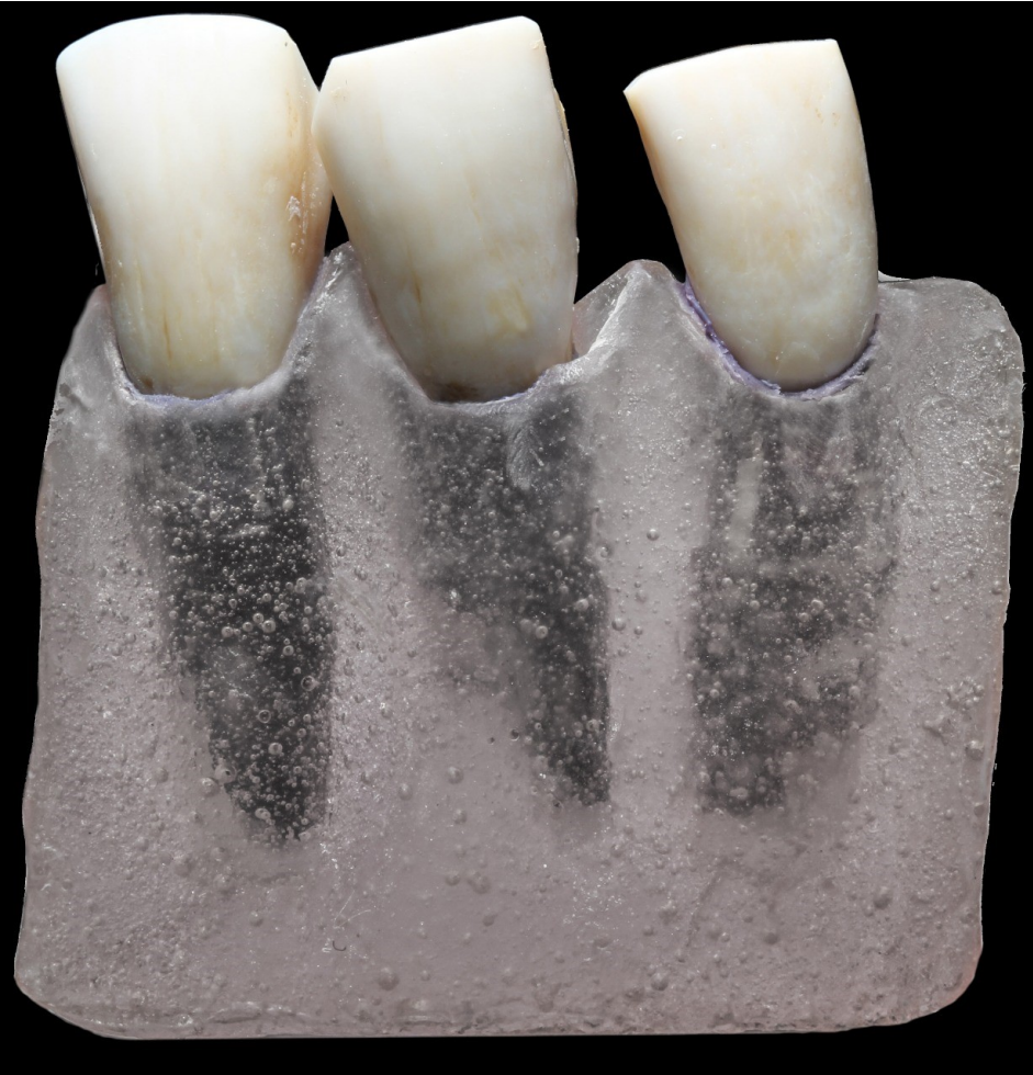
Fig. 1. Artificially created model to simulate the anterior mandible region, with three dental alveoli: one central socket for the tooth to be analyzed (root fracture) and two adjacent sockets for sound teeth.
