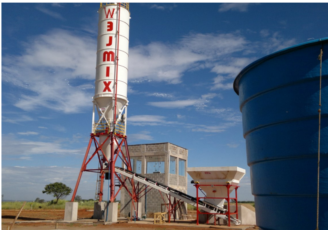
Figura 7- Central dosadora de concreto Tow Go
