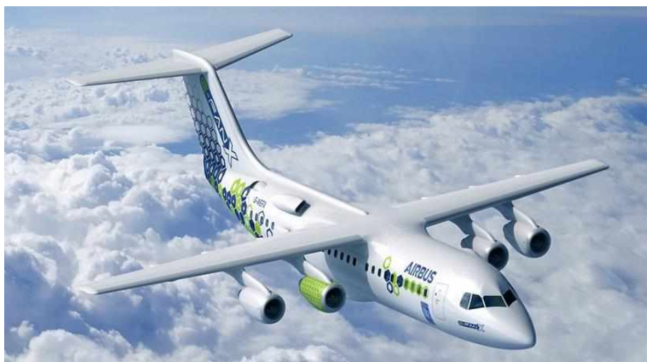
Figure 2 – Airbus E-Fan X: a hybrid-electrical aircraft demonstrator.
