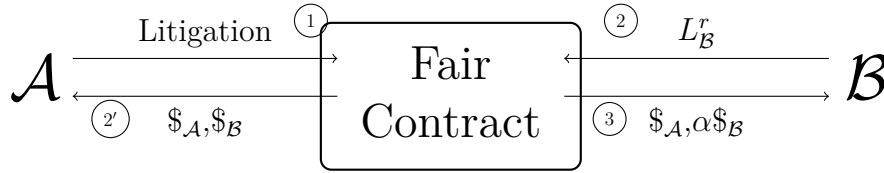
Figure 6 – FairContract in litigious mode. \mathcal{B} sends L_{\mathcal{B}}^r to FairContract and receives the payment. If not, after a timeout, \mathcal{A} receives the contract values.
