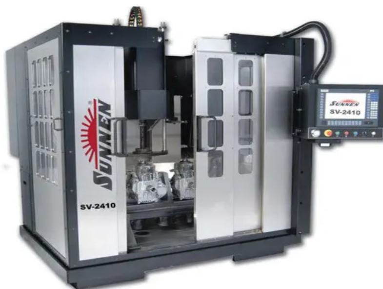
Figura 16: Brunidora tipo honing vertical SV-2400 series (DIRECT INDUSTRY, 2020).
