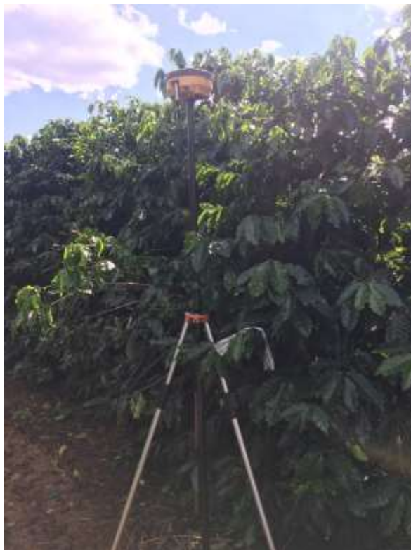
Figura 7 - Receptor GNSS RTK
