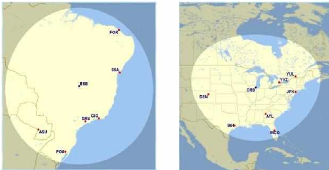
Figure 27: Range of the 4PAX aircraft from Brasília (on the left) and Chicago (on the right).
