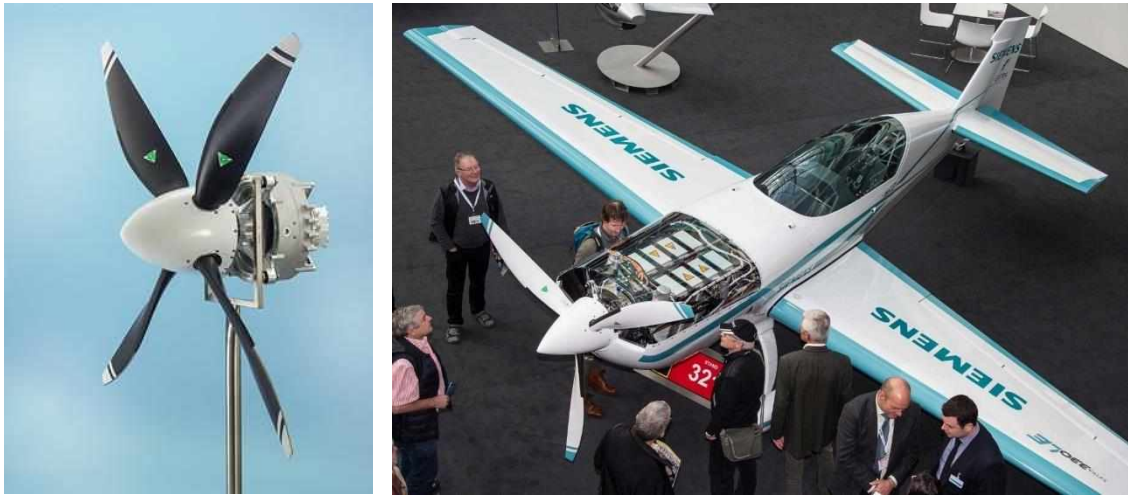
Figure 5: Electric motor SP260D (on the left) and Siemens Extra 330LE (on the right). Source: Endless Sphere.
