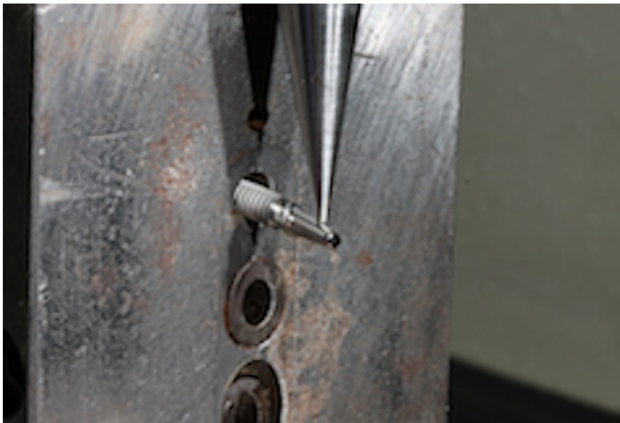
Figure 3 – The implant and the metallic holder were fixed on the mechanical testing machine (EMIC; 2000DL) and submitted to a load cell of 500 KN capacity (KN500; EMIC).
