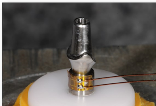
Figure 4 – Strain gauge fixed in the cervical portion of the implant. Note that the implant was fabricated without external threads to permit this fixation.
