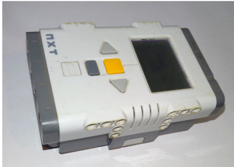
Figura 3.7 – CLP (ou intelligent brick ) do kit LEGO Mindstorms NXT ® .
