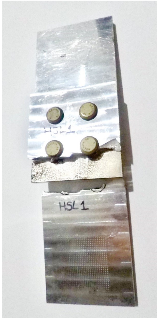
Figure 71 – HSL1 after rupture. Source: author.
