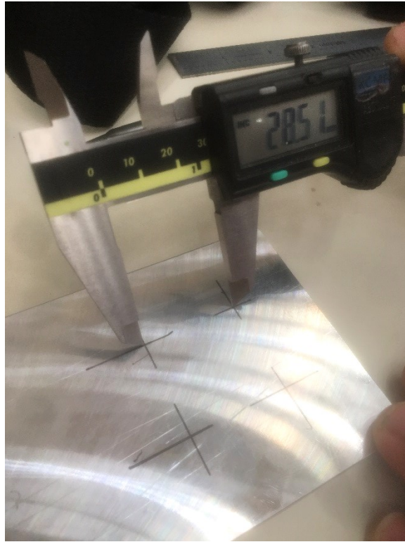
Figure 55 - Plates marking and measurement. Source: author.
