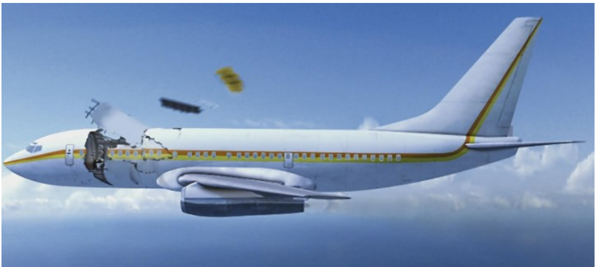
Figure 39 – Overload separation during Aloha Airlines Flight 246. Source: Seelio, 2016.
