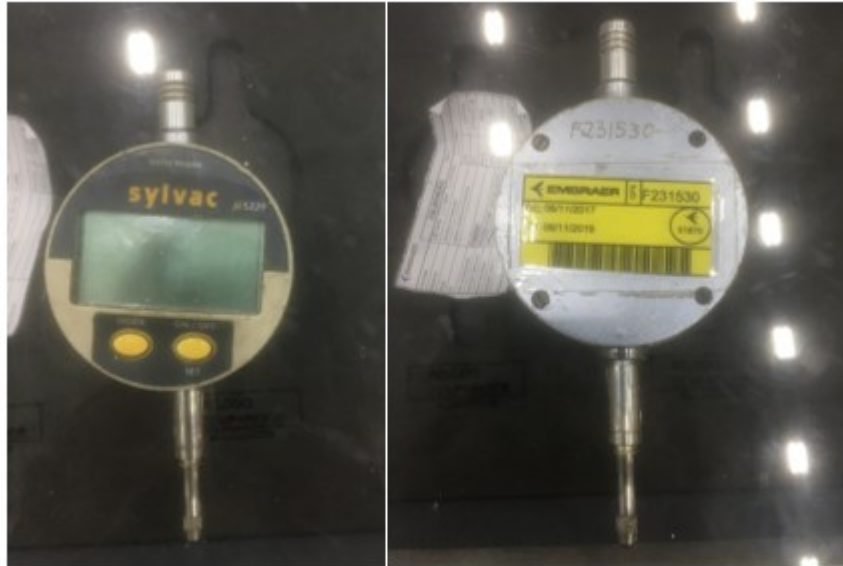
Figure 58 - Comparator used to measure the holes diameter. Source: author.
