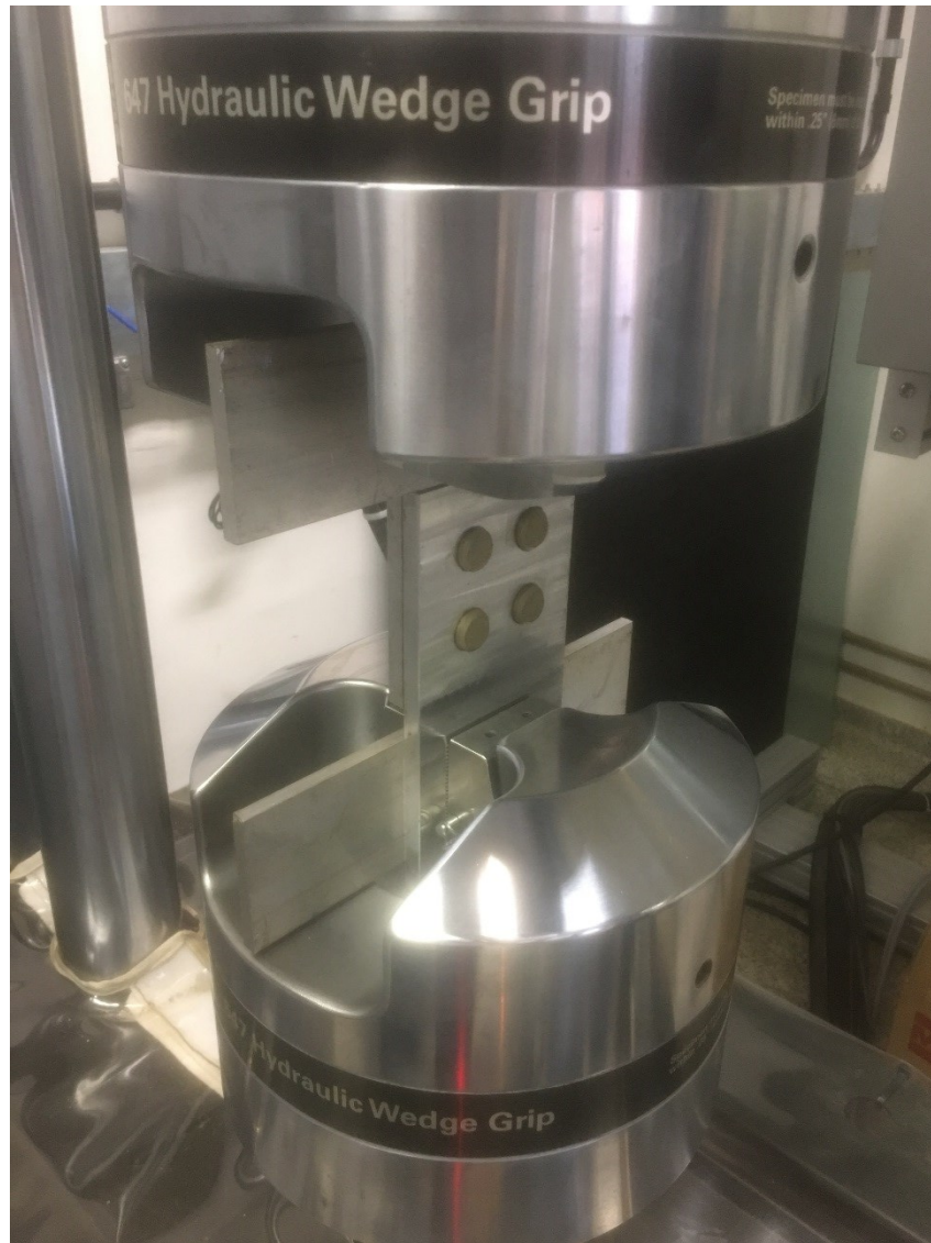
Figure 68 – Sandwich assembly on MTS machine. Source: author.
