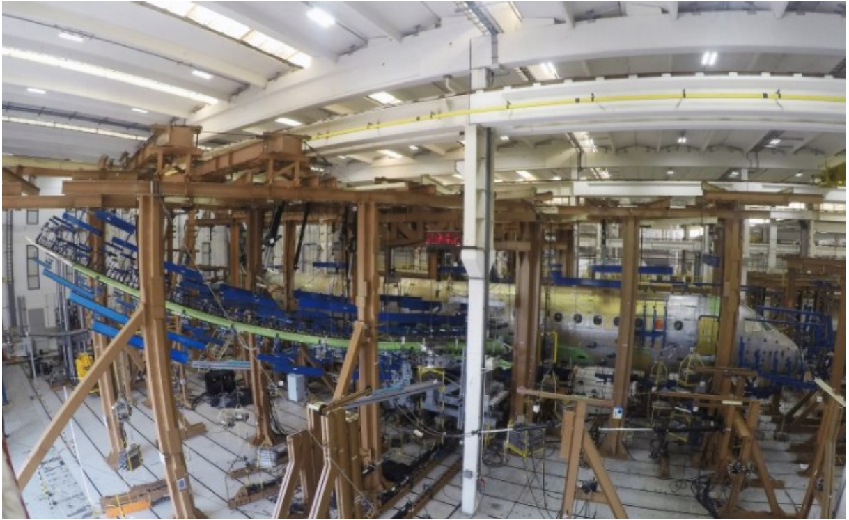
Figure 37 - Embraer E190-E2 certification ultimate load fatigue test. Source: EMBRAER, 2017.
