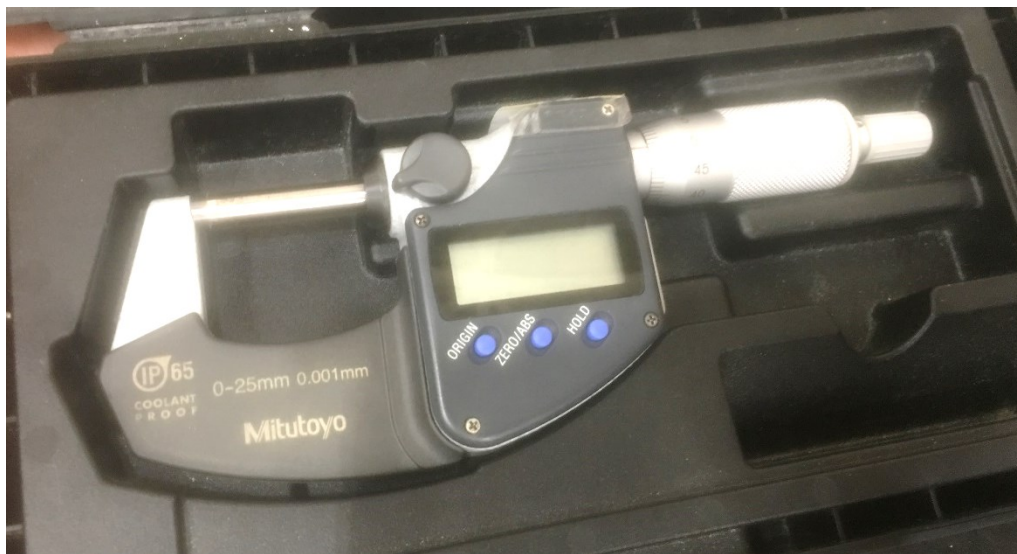
Figure 61 - Micrometer used to measure the pins shank diameter. Source: author.
