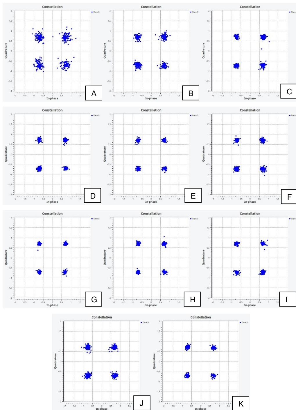
Figura 38 – Constelações canal 28. (A) -105dB, (B) -102dB, (C) -99dB, (D) -96dB, (E) -93dB, (F) -90dB, (G) -87dB, (H) -84dB, (I) -81dB, (J) -78dB, (K) -75dB.
