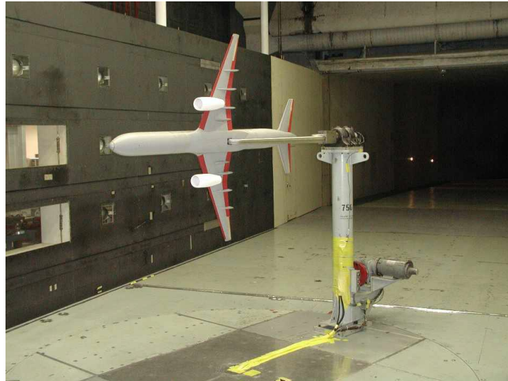
Figure 3-5 Roll forced oscillation rig, NASA LaRC 14x22 ft Tunnel
