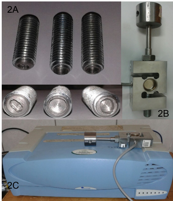
Figure 2. 2 A: Implant heads. 2B: Load cell in instruments. 2C: LYNX acquisition system.
