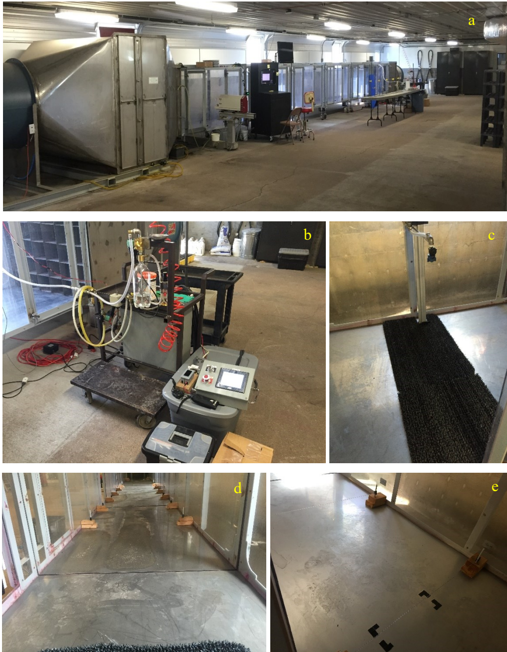
FIGURE 1A. Wind tunnel facility: structure of the tunnel (a), spraying controller (b), spray zone (c), and positions of drift collectors (d and e).
