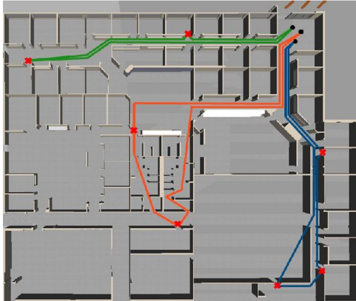
Figure 1 – Coordination : route scheduling. This figure illustrates the scenario where the routes (colored lines) of 3 robots (black dots) cover all desired locations (red crosses) of the environment.
