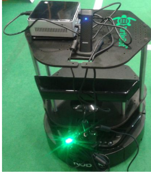
Figure 25 – Turtlebot 2: robotic platform used in our indoor localization experiments with Kinect and WiFi devices.
