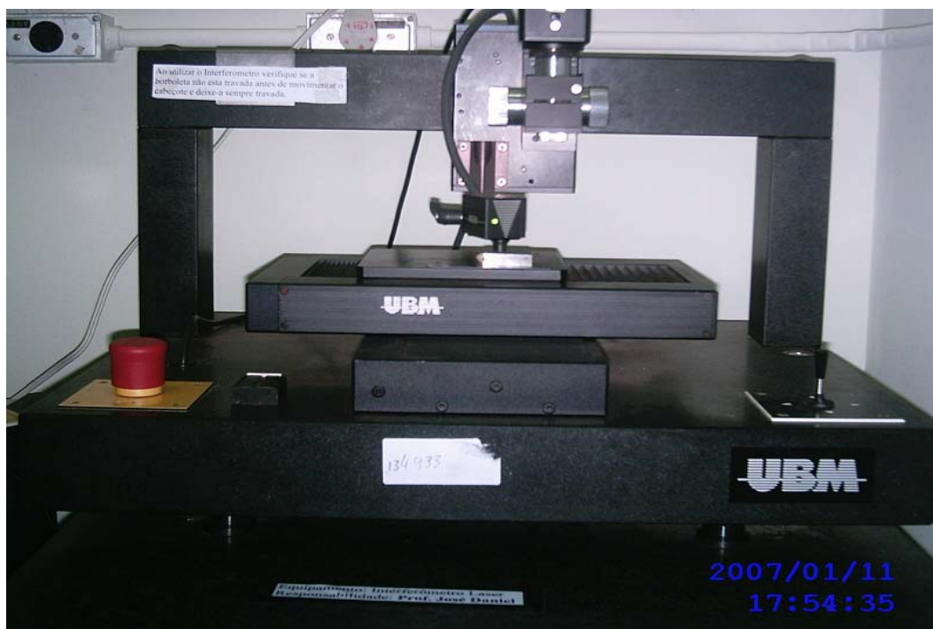
Figura 15. Interferômetro a laser 3D modelo microfocus expert, marca UBM
