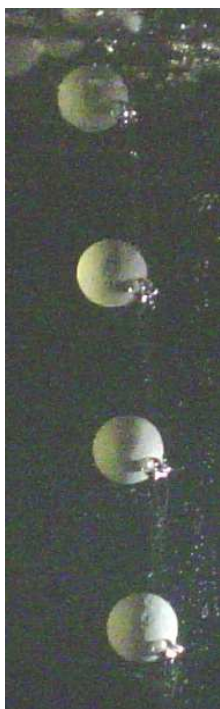
Isopor 6T ( \rho_s = 0,107\text{g/cm}^3 ; d_{\text{médio}} = 3,421\text{cm} ).
