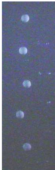
Isopor 1T ( \rho_s = 0,594\text{g/cm}^3 ; d_{\text{médio}} = 1,508\text{cm} ).
