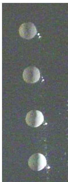
Isopor 3A ( \rho_s = 0,362\text{g/cm}^3 ; d_{\text{médio}} = 2,440\text{cm} ).
