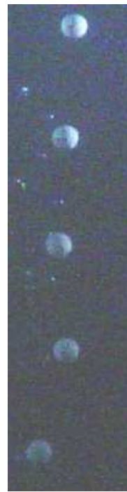
Isopor T ( \rho_s = 0,562\text{g/cm}^3 ; d_{\text{médio}} = 1,475\text{cm} ).
