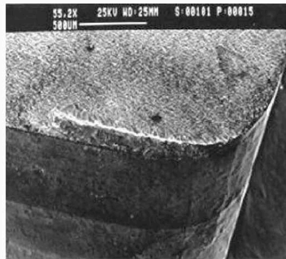
Figure 2.37 - Formation of strongly adherent layer on the rake face of a PCD tool after machining titanium base, Ti-5Al-4Mo-2Sn-6Si alloy under dry condition (NABHANI, 2001b).
