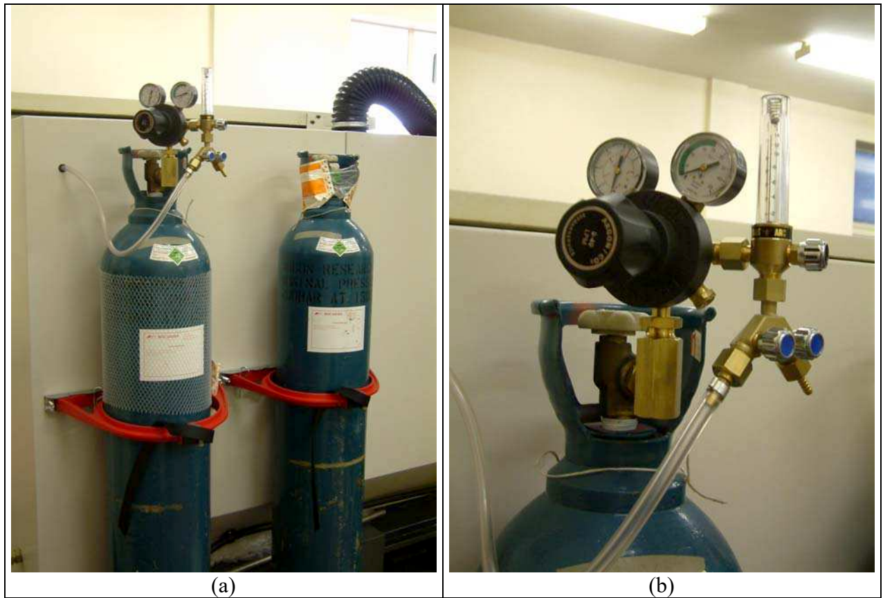
Figure 3.4 - Argon gas delivery system: (a) cylinder and (b) close-up view of the valve and the hose.
