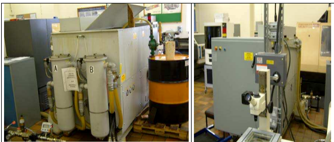
Figure 3.2 - The high pressure pumping coolant system - Chipblaster (CV26-3000).
