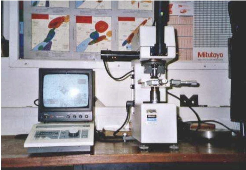
Figure 3.12 -Mitutoyo (MVK – VL) Vickers micro-hardness tester machine.
