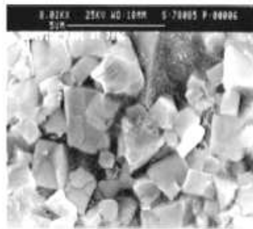
Figure 2.30 - SEM micrograph of exposed mixed cemented carbide substrate after fracture of the welded junction (NABHANI, 2001b).
