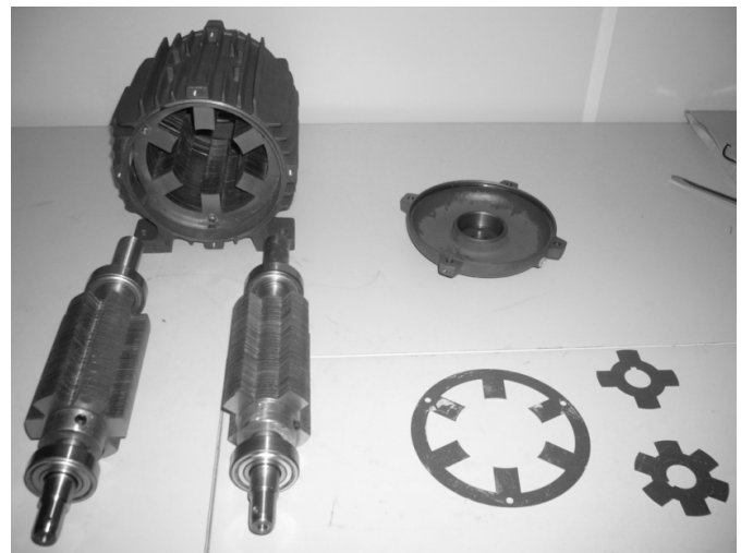
Fig. 3. Parts of a prototype of Switched Reluctance Generator.
