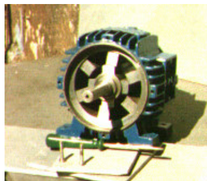
Fig. 2 – Picture of the SRG prototype constructed.
